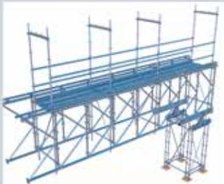
**Scaffold bridge** – K-Frame as the basis for your modular or façade scaffolding saves an enormous amount of time and material quantities. Ideal when the supporting surface is not as it should be.
