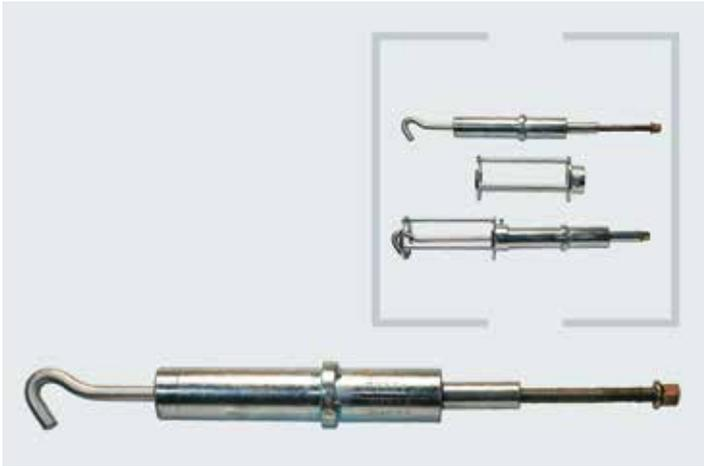
**Anchorage testing device**
