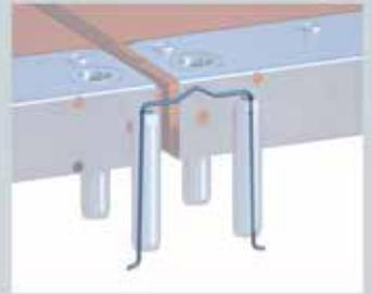
**Safe** – Decks are secured against lift either by the integrated deck retainers or by retaining springs (Art. No. 04552) in the case of system decks.
