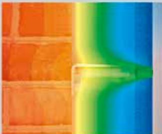
**Stainless steel** – The VA stainless anchor remains permanently in the façade and – unlike most solutions offered – features minimal thermal conductivity.
