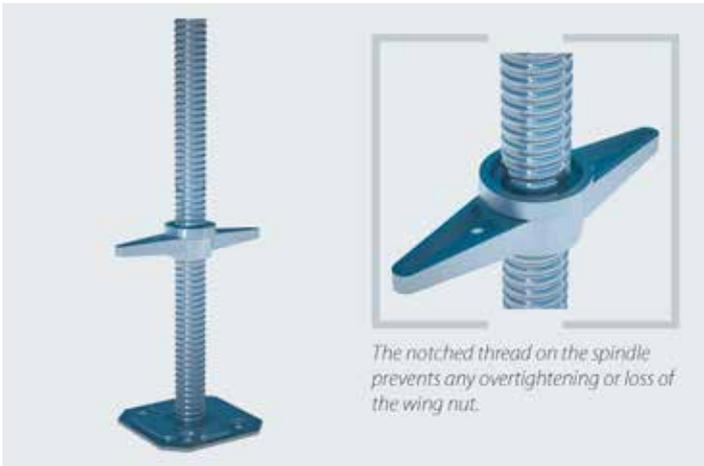
The notched thread on the spindle prevents any overtightening or loss of the wing nut.
