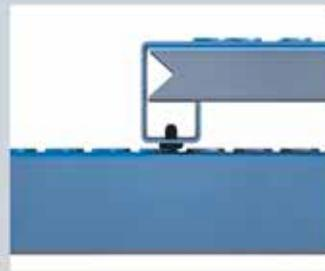
**Secure** – When scaffolding is installed inside buildings, additional securing of the decks is frequently unnecessary.
